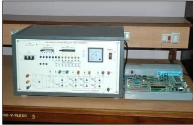
**IPM Power Module with DSP Controller**
