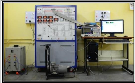
**Three Phase Seven-Level Neutral Point Clamped Inverter**
