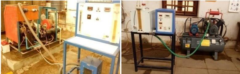
Multi cylinder 4 stroke petrol engine test rig Air Compressor Test Rig
