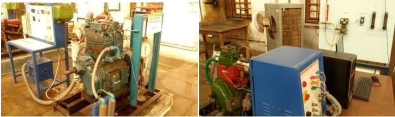
Variable Compression Engine test rig Twin cylinder 4 stroke diesel engine test rig
